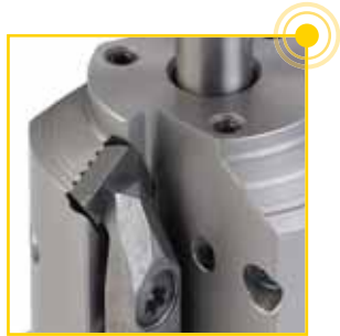
RIQ serration defines valve seat angle
