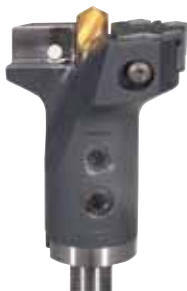
Pilot drill should be installed and set to the proper length before installing the inner cartridge.
