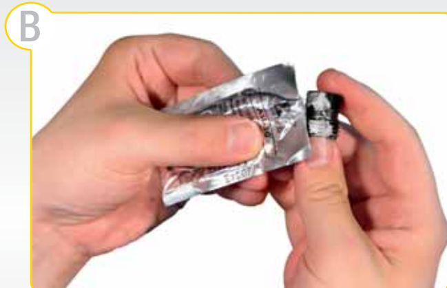
B. Lubricate the thread on the Differential Connector (5) with Lubricant ASL-3G (7), supplied with the Taper Shank (2).
