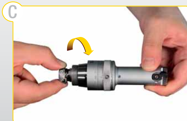
C. Screw the Differential Connector (5) into the rear thread on the Boring Head (1) until the end of the thread. At this time it is not necessary to tighten the Differential Connector (5). Remember that the Differential Connector (5) has two different screws, so there is no way to assemble the wrong side.
