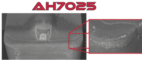
Tool wear after 60 grooves
