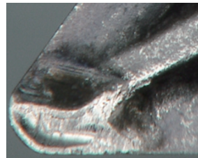
Excessive crater wear with external coolant supply (at normal pressure)
