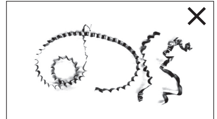
Continuously coiled long chips
